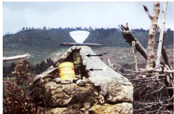
Fig. 2. Cross-section of rain gauge (Harena-Argaka). Note the two metal tins fixed in cement (arrows), which hold a plastic bottle with funnel (diameter = 12.7 cm).
